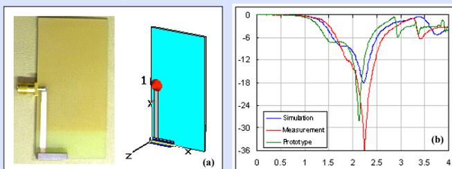
Fig. 5. (a) Photo and Model of the optimised design (b) Return losses for simulated prototype antenna, simulated optimised antenna and measured optimised antenna
