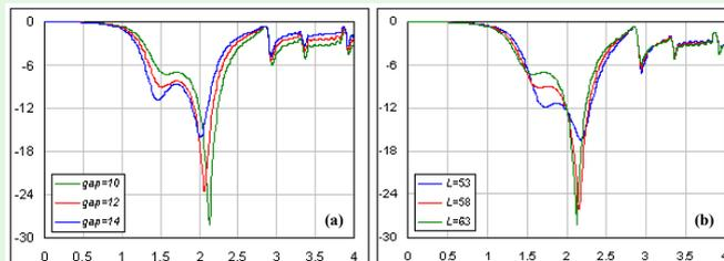
Fig. 4. (a) Return losses for antenna with different gap (10mm-14mm) (b) Return losses for antenna with different L (53mm-63mm)
