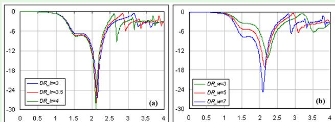
Fig. 3. (a) Return losses for antenna with different  $DR_h$  (3mm-4mm) (b) Return losses for antenna with different  $DR_w$  (3mm-7mm)
