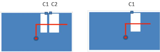
**Fig. 1:** Starting points. Two capacitively loaded notches fed in series by a microstrip line (left) and a single loaded notch fed by a microstrip line (right). The antennas were constructed on 0.8-mm thick FR4 with the groundplane and notch on one face and the feed on the other face.
