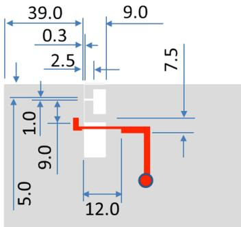
Fig. 7: A single loaded notch providing pentaband coverage. The feed track is 2.5 mm wide except for the section across the notch which is 1.3 mm wide.
