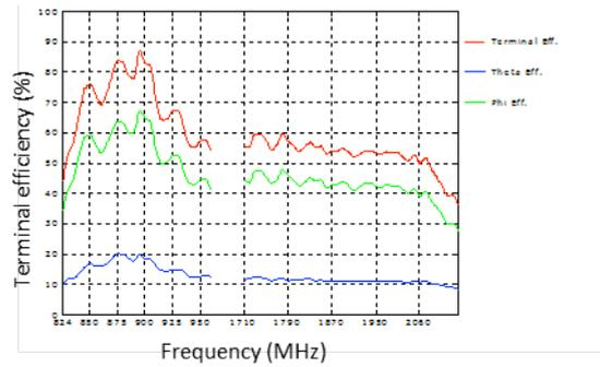
**Fig. 3:** Measured terminal efficiency of the antenna shown in Fig. 2.
