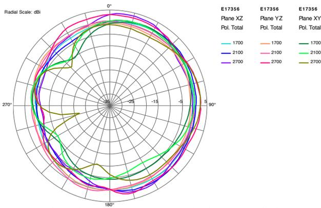
Fig. 6: Dual notch 23mm x 23mm. Polarization sum radiation patterns at 1700, 2200 and 2700 MHz. The PCB lies in the x-y plane with its long axis along the 0/180 degree axis.
