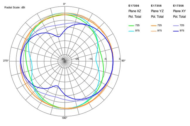
**Fig. 5:** Dual notch 23mm x 23mm. Polarization sum radiation patterns at 725 MHz and 960 MHz. The PCB lies in the x-y plane with its long axis along the 0-degree axis.
