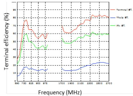
**Fig. 4:** Terminal efficiency of 23 mm x 23 mm multi-band dual notch on a PCB 133 mm x 60 mm.
