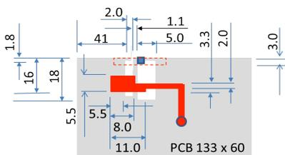
The copper strip indicated by a dashed rectangle is 17.1 long and overlaps the groundplane by 6.0mm at its right hand end
