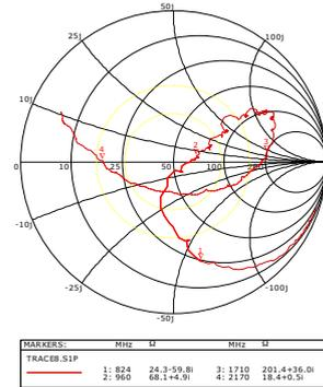
Fig. 9: Smith chart plot of the impedance of the single notch pentaband antenna at the coaxial input connector with no added matching network.
