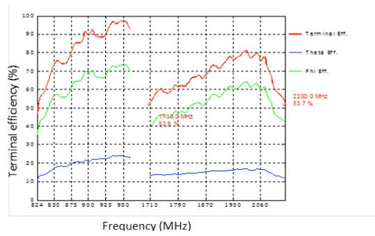
Fig. 8: Terminal efficiency of the single 27 mm x 9 mm pentaband notch illustrated in Fig. 7.
