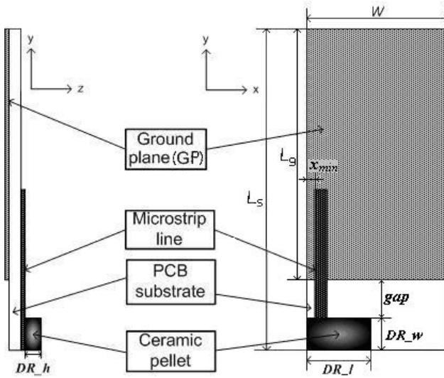
Fig. 1. Geometry of the prototype antenna
