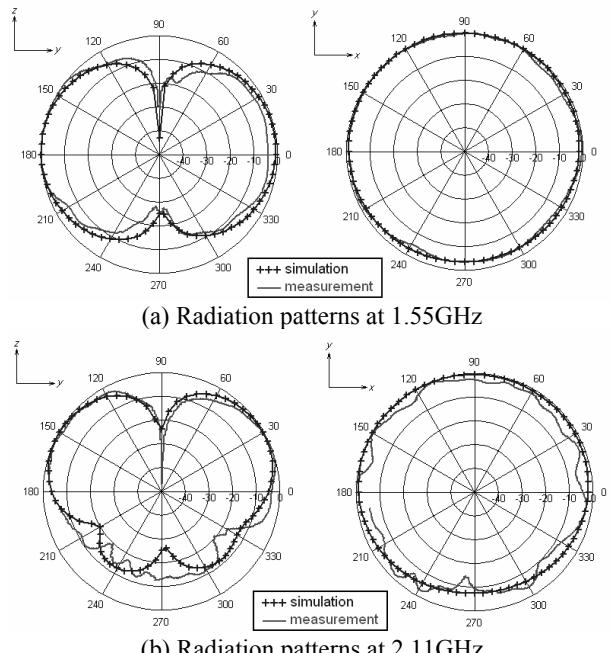
Fig. 3. Simulated and measured radiation patterns of the prototype antenna
