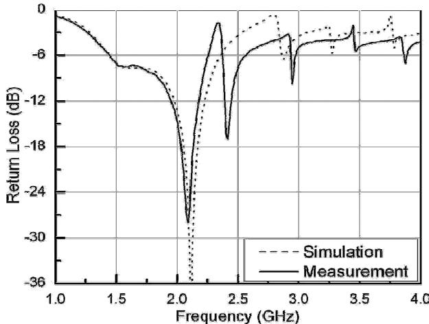
Fig. 2. Simulated and measured return losses of the prototype antenna
