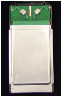
Figure 7. Two dual-band WLAN antennas covering the 802.11a&b bands on a PCMCIA card
