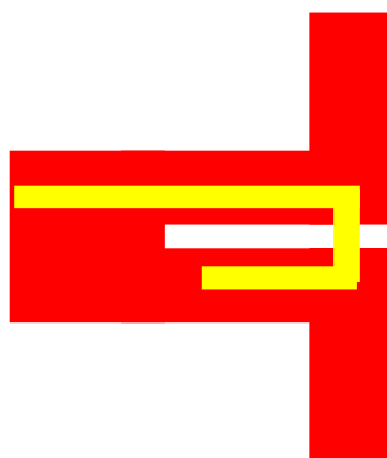
Figure 8: A Roberts 'hairpin' balun applied to a microstrip dipole
