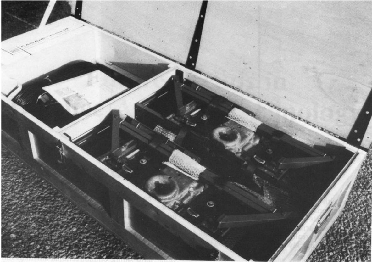
*Using an active receiving array, a high performance antenna is reduced to a compact boxful.*
