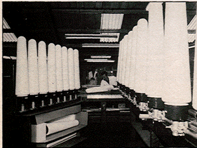
3 Slow-wave antenna for low-capacity subbands prepared for inspection prior to despatch
