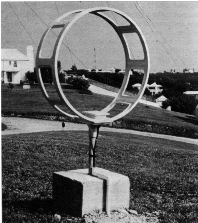
Active loop receiving antennas using fibreglass-encased conductors to avoid corrosion
